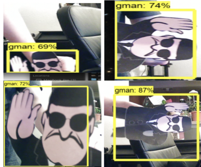
Fig. 14. Confidence level increases after training with a larger data set.
