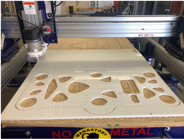
Fig. 8. HDPE frame being cut on a CNC router.
